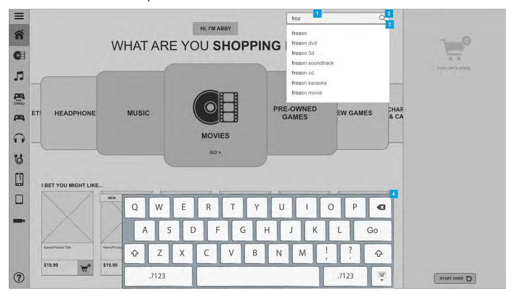
On tap of the search box, the keyboard is shown to allow the user to enter search keywords. The user can hide the keyboard by tapping outside of it or hitting "Go" to complete the search.
